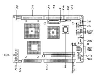
Figure 2.1: Jumper & Connector Locations
